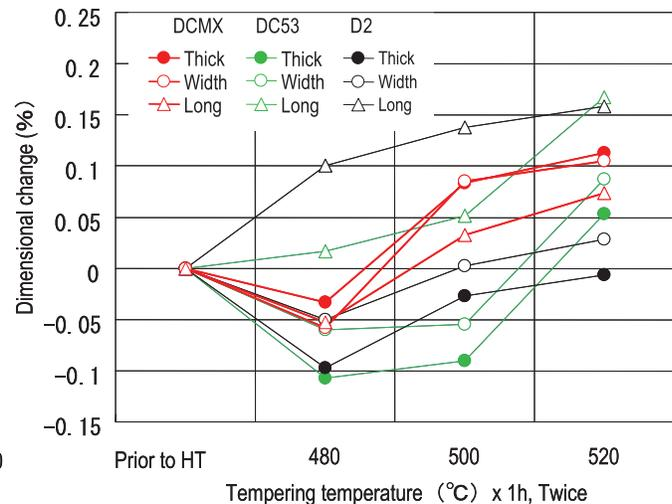
Specimen: 50mm Thick x 100mm Width x 150mm Long
